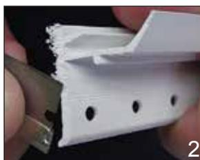
2. Remove frays left by the saw blade after cutting.
